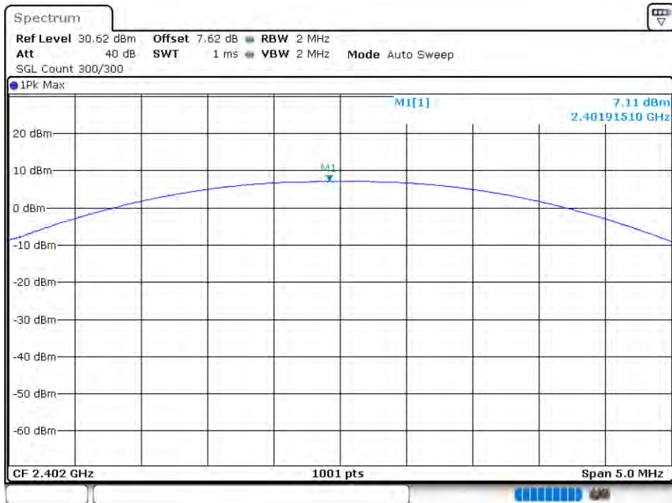
Power NVNT 1-DH5 2402MHz Ant1
