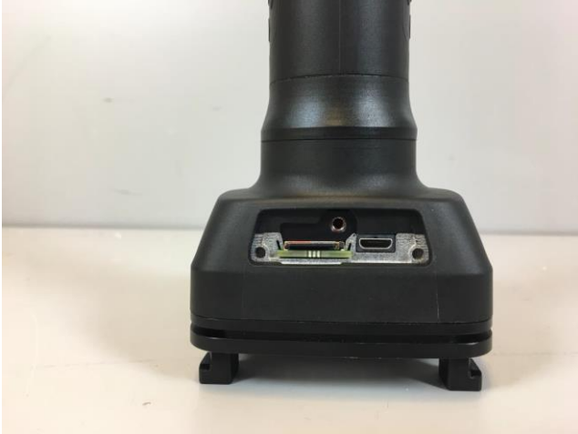
View of tool without lid and exposed USB port and SD card slot
