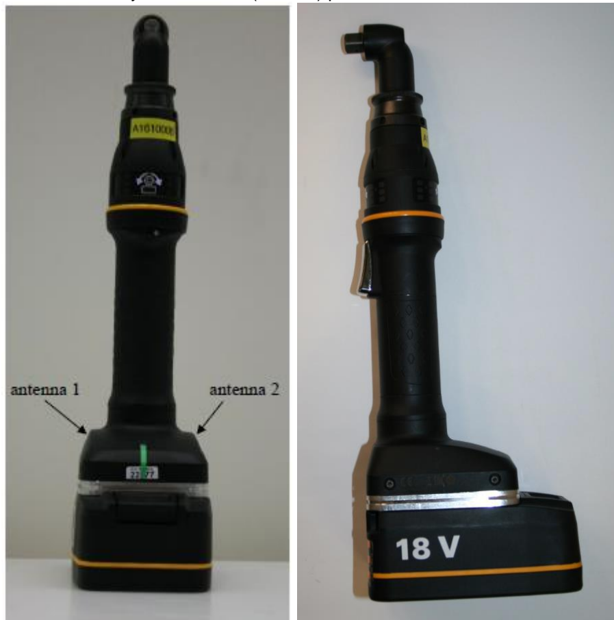
View with battery and antenna (internal) placement
