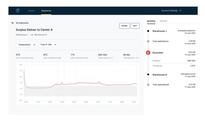
You can see your shipment data overlaid on top of your expected ranges (shown in grey) as an option for your graph display. Additionally, all thresholds breached in transit are listed as excursions in the Activity Feed on the right-hand side of the screen.
