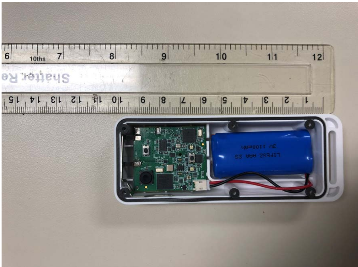
Figure 2 - Parsyl Trek - Internal View – PWB & Battery in Case with scale
