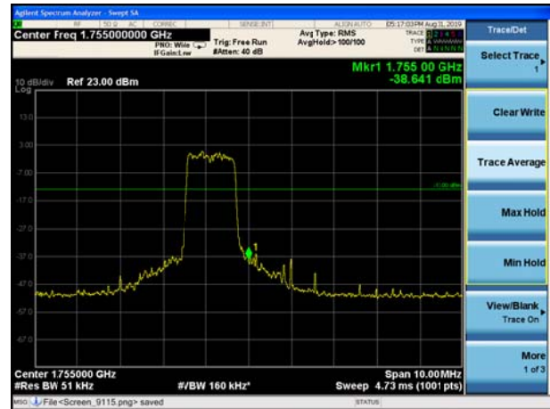
LTE Band 4 QPSK 5MHz CH-High, 1 RB
