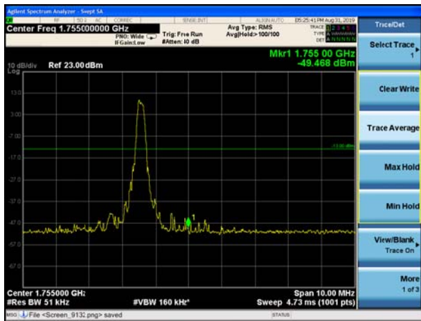
LTE Band 4 16QAM 20MHz CH-Low, 100%RB
