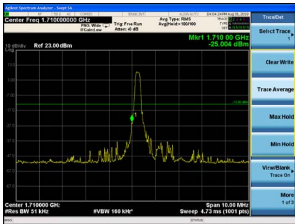
LTE Band 4 QPSK 1.4MHz CH-Low, 100%RB
