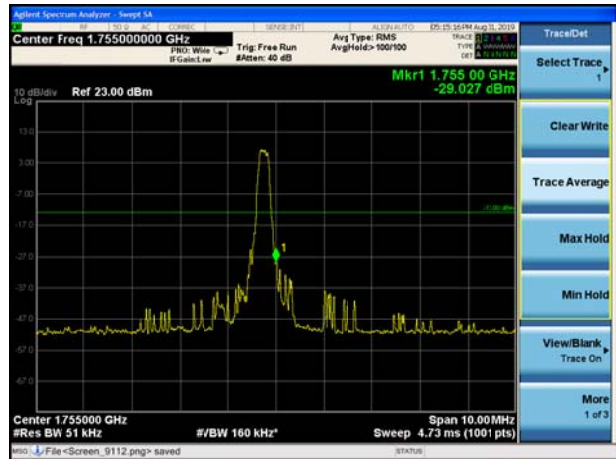
LTE Band 4 16QAM 1.4MHz CH-High, 100%RB
