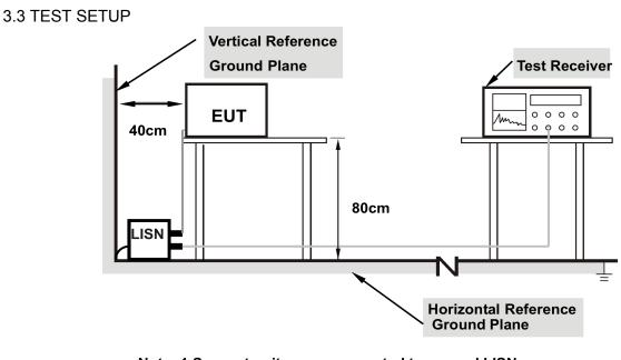
Note: 1.Support units were connected to second LISN. 2.Both of LISNs (AMN) are 80 cm from EUT and at least 80 from other units and other metal planes
