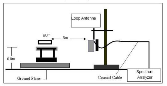
(B) Radiated Emission Test-Up Frequency 30MHz~1GHz
