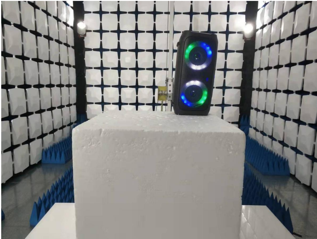
Blow 1GHz for radiated emission test setup
