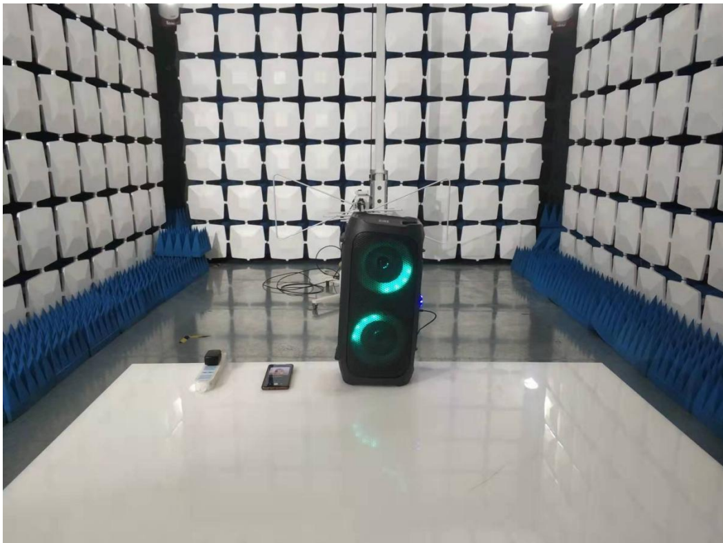
Blow 1GHz for radiated emission test setup
