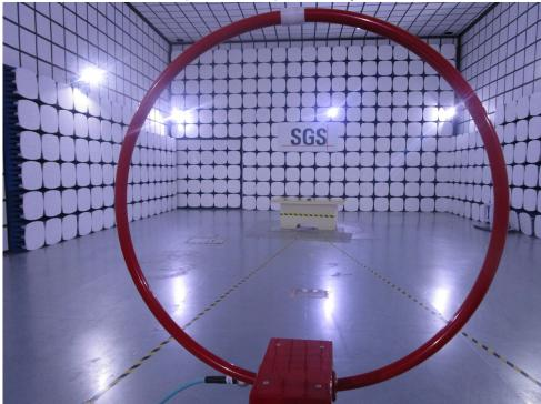
1.2 Radiated Emissions(30MHz-1GHz) Test Setup
