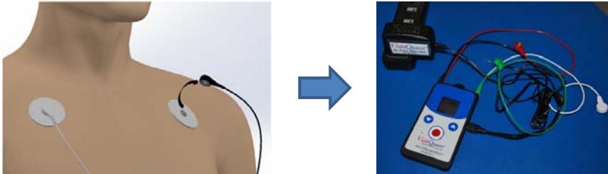
Remove leads from electrodes then plug RX-1 into charger.
