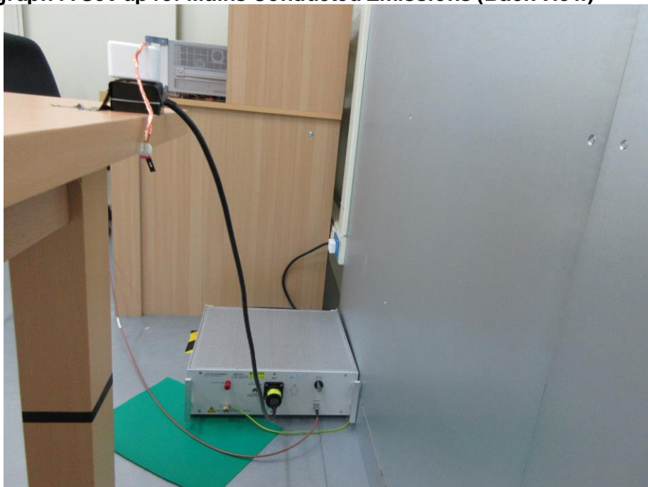
Photograph 7: Set-up for Mains Conducted Emissions (Back View)
