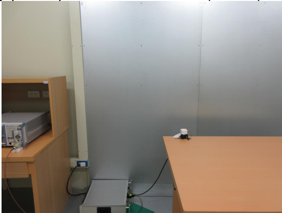
Photograph 7: Set-up for Mains Conducted Emissions (Back View)
