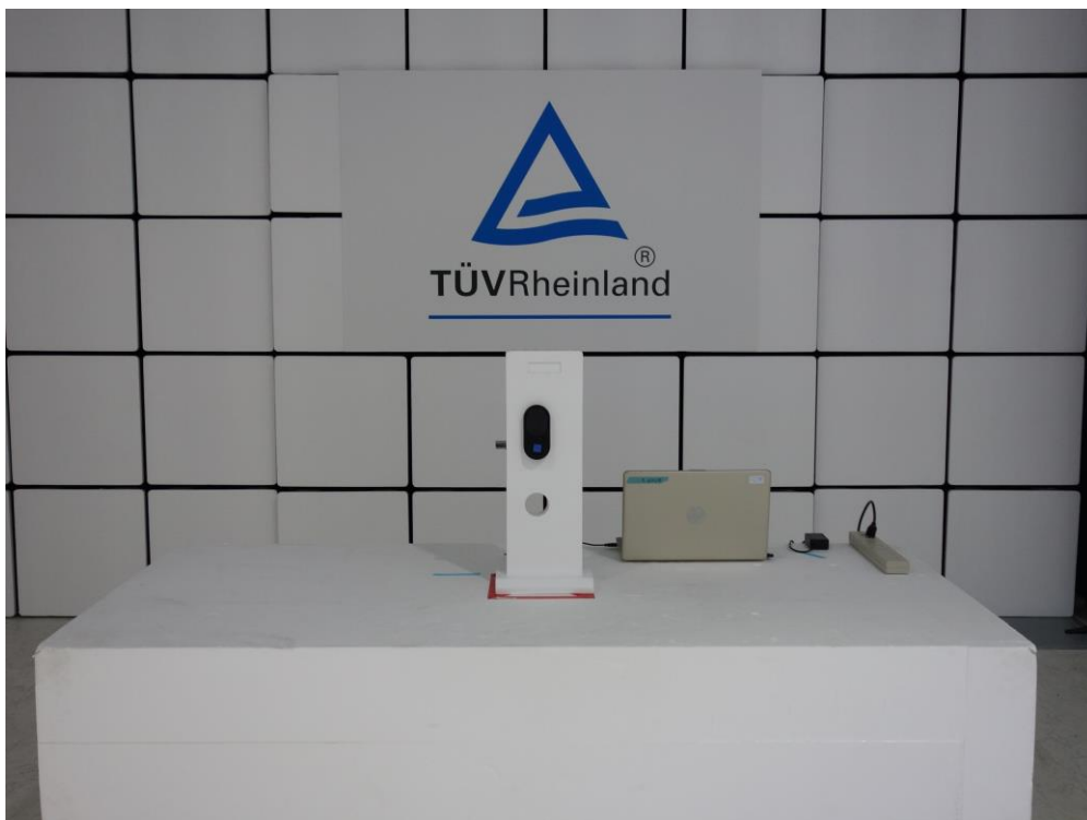
Photograph 2: Set-up for Spurious Emissions (Front View 2)
