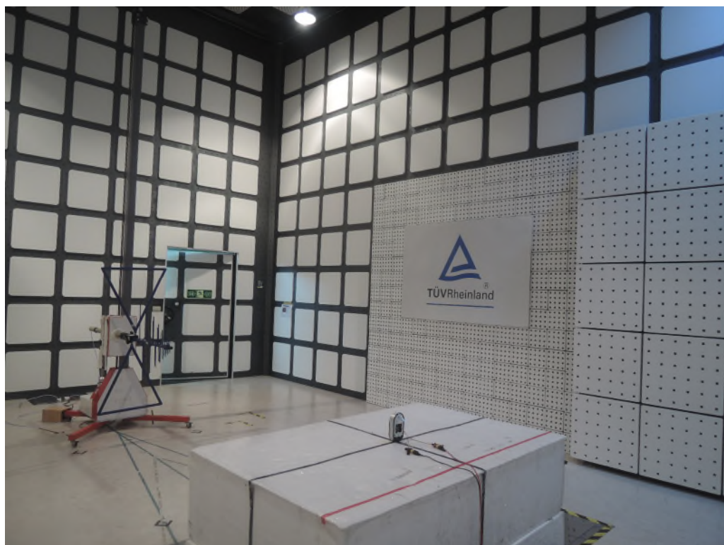
Photograph 2: Set-up for Radiated Emissions (Back View 1)
