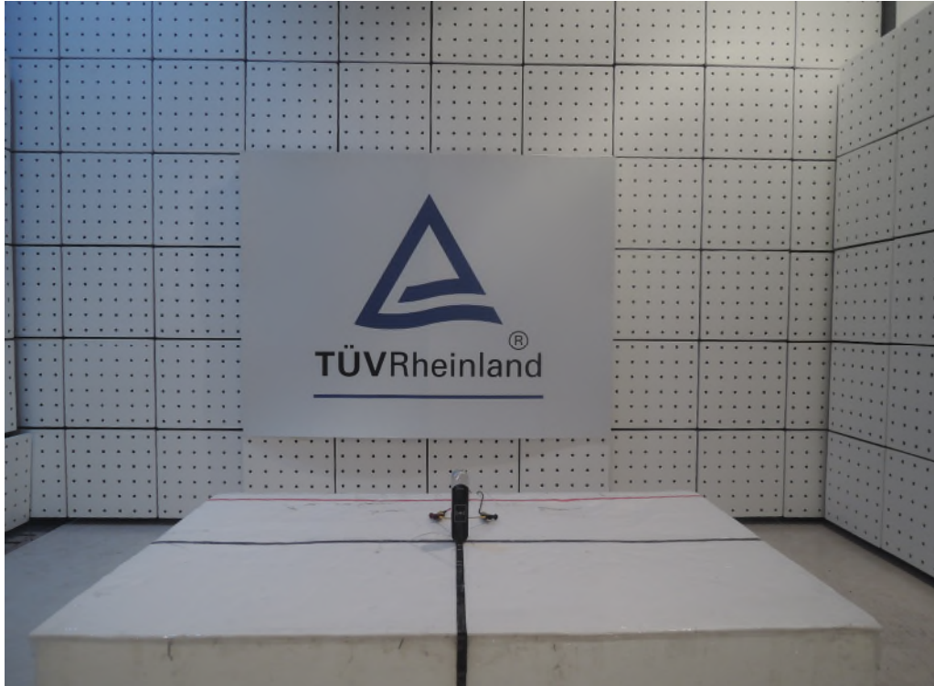
Photograph 2: Set-up for Radiated Emissions (Back View 1)
