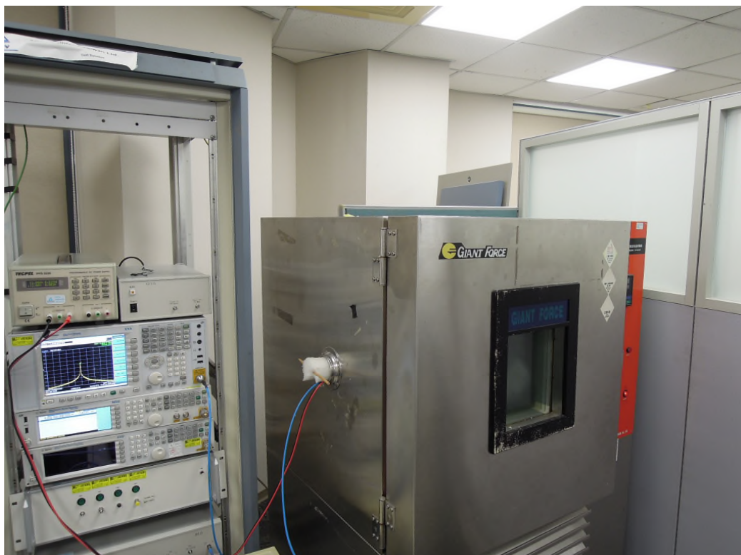
Photograph 4: Set-up for for Conducted testing
