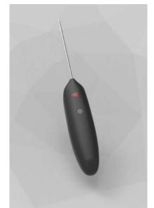
The Handheld Temperature Probe is developed to perform a manually triggered temperature measurement activity of the desired zone or touched product. By pushing the button, the probe will be activated and start the measurement. After 5 seconds of stabilized contact, the temperature figure collected will be send to the server using IEEE 802.15.4 communication protocol.
