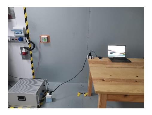
Set-up for Radiated Emission (RE), Below 1GHz
