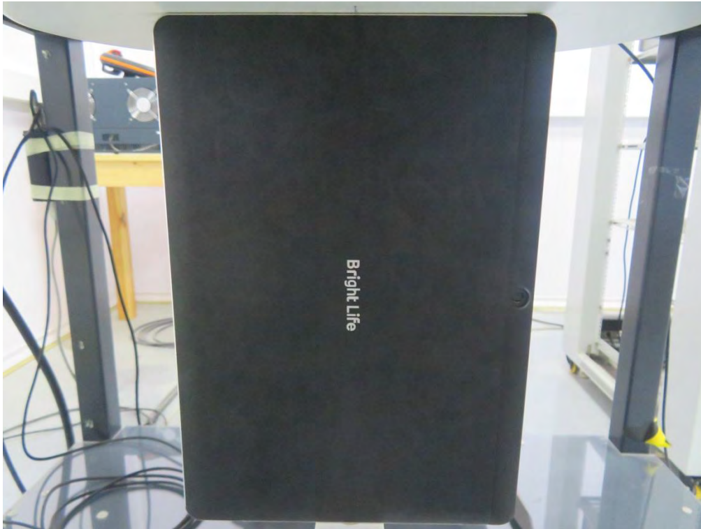
0mm body-worn Right Side Setup Photo (hotspot)
