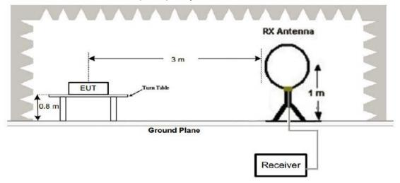
(2) Radiated Emission Test-Up Frequency 30MHz~1GHz
