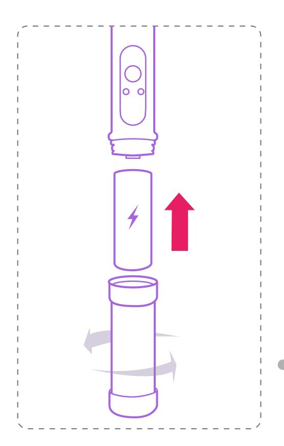
Rotate to loosen the end cover, then install a 18650 Li-ion battery (with the positive pole heading in the same direction as the arrow above). Make sure to tighten the end cover properly after battery installation, or the TaroVR Bot cannot be turned on.
