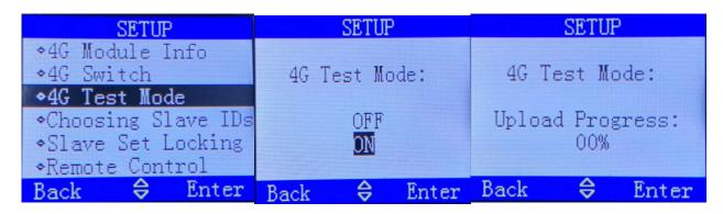
4G Test Mode is for 4G upload testing. When you choose this option and select on, it will automatically upload a photo to server. And you can see the Progress on Screen.
