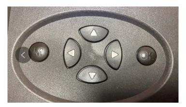
M button is for enter the menu setting ,press the menu button, the camera will enter the menu setting interface (as shown below)
