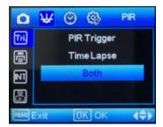
Press the ▼ button to highlight the **Trigger Mode** option in blue. Under this setting you can choose **PIR Trigger** (Where the camera is triggered by heat or motion only), **Time Lapse** (Where you tell your camera to take pictures every 5 seconds up to 24 hours) or **Both**. Highlight your selection and press **OK**. Press the **Menu** button to go back to the previous screen.
