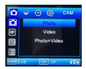
Under the Camera Mode tab, select whether you want Photo, Video or Picture+Video. Press **OK** to save. Press **MENU** to go back to the Camera Mode and **Customize** screen. Press the ▼ button one time until **Customize** is highlighted in blue. Press **OK**. If you chose Photo or Picture+Video Video Size and Video Length will show up. Under the **Customize** menu, press the ▶ button to change the photo size. You may choose between: 3MP, 5MP, 8MP, 10MP, 12MP..up to 32MP
