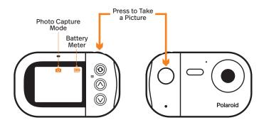
Press the Power/ OK button 1 or Shutter release 2 to take a picture.
