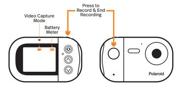
Press the Power/ OK button ① or Shutter release ② to begin recording video. Press it again to end your recording
