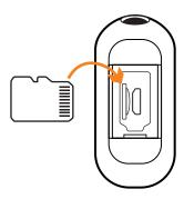
Before turning on your camera, insert a Micro SD memory card (NOT included) into the **memory card slot** ②. The memory card is needed in order to store photos or videos.
