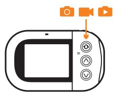
Once the camera is powered on, press the **Mode / Menu button ②** repeatedly to switch between the camera's different modes.
