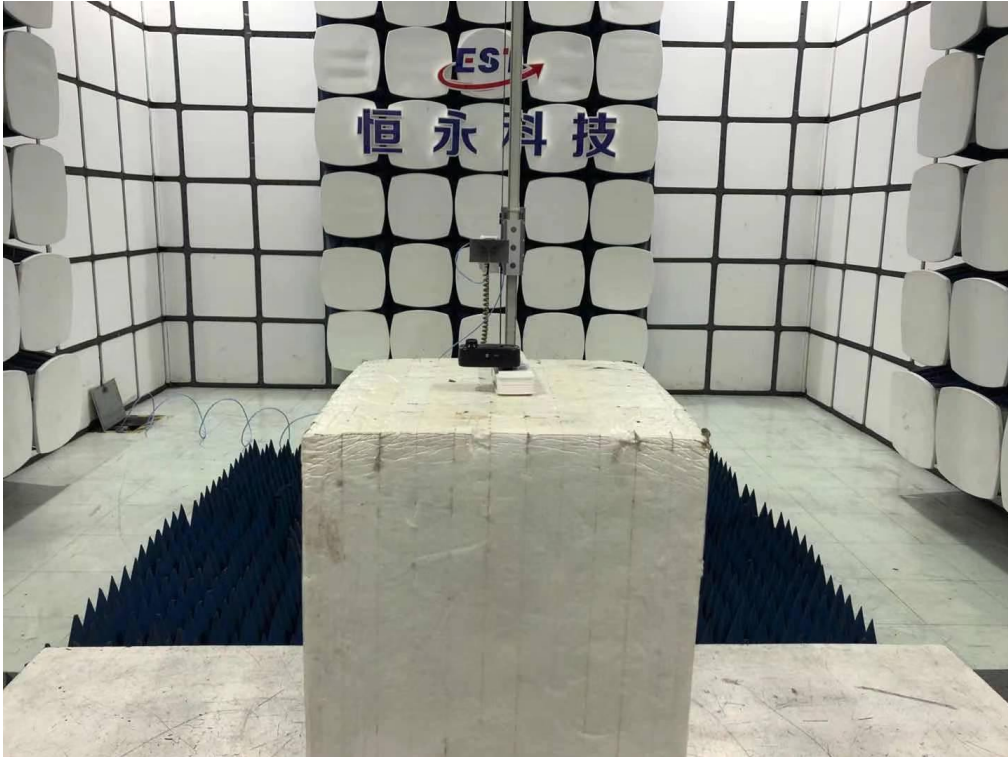
Radiated Test (Above 1GHz)
