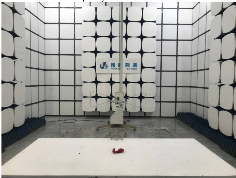
Radiated Spurious Emissions Test Frequency From 30MHz-1000MHz
