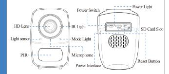
How to reset camera: When the camera is turned on, press and hold the reset button for about 3 seconds until you hear the "reset complete, will restart the device" or the blue light and green light flash slowly at the same time, and then the blue light flashes slowly.
