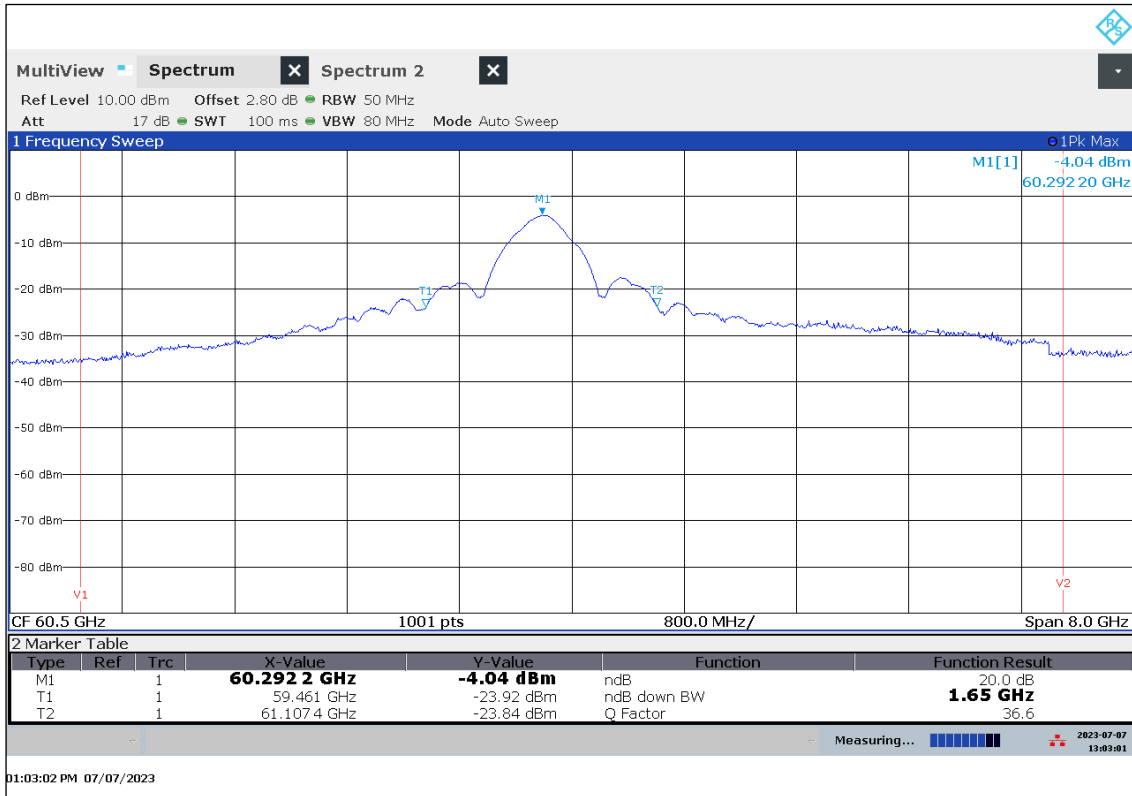
Plot 27: 20 dB-Bandwidth at T= 50 °C / V min-max
