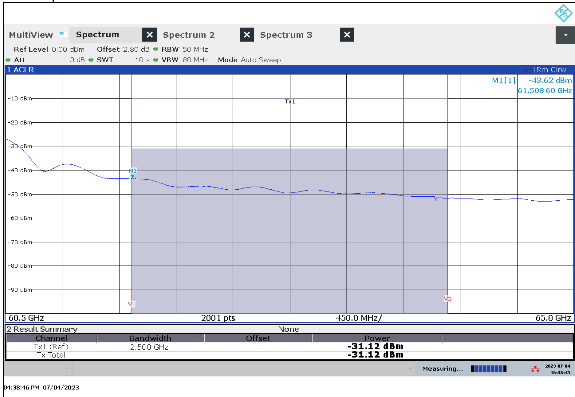
Plot 6: Channel power within 61.5 to 64 GHz without lens
