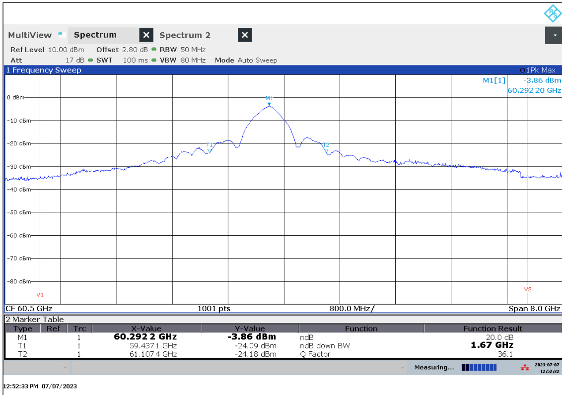
Plot 28: 20 dB-Bandwidth at T= 85 °C / V min-max
