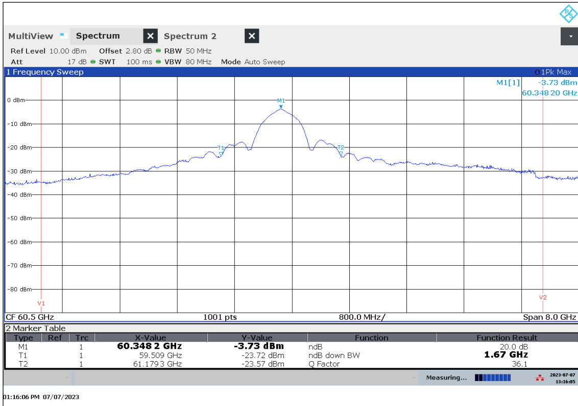
Plot 25: 20 dB-Bandwidth at T= 30 °C / V min-max
