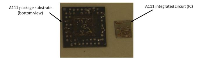
External pictures: A111 radar sensor - top and bottom view:
