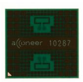
Top view of A111 package substrate with integrated antennas
