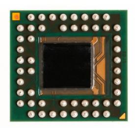
Figure 2, Backside of the A111 sensor.
