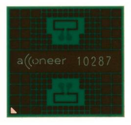
Figure 1, Frontside of the A111 sensor.
