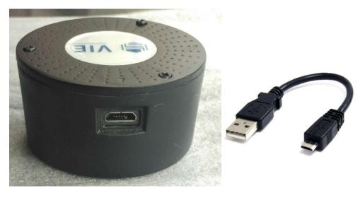
STEP 1: Connect the modified micro USB to USB cable, supplied by VIE Technologies, to the MyVIE Spin.
