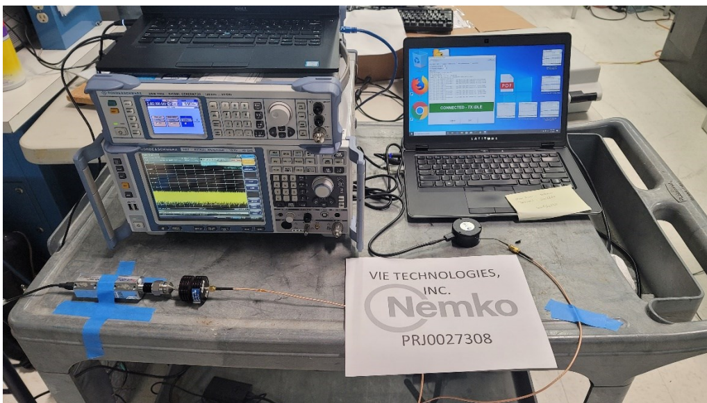
Figure 6 – Test setup: power meter, antenna conducted port.
