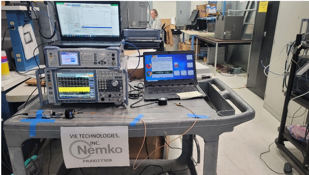
Figure 5 – Test setup: power meter, antenna conducted port.
