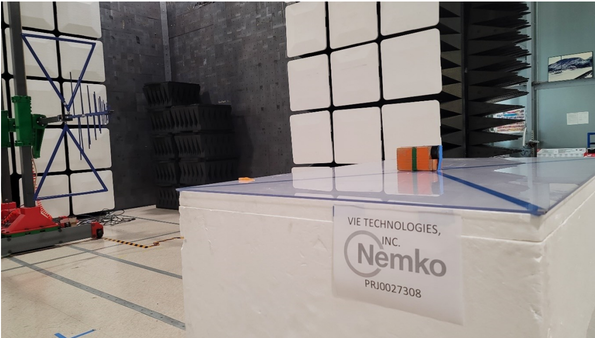
Figure 2 - Radiated emissions below 1 GHz (0.03 – 1 GHz).
