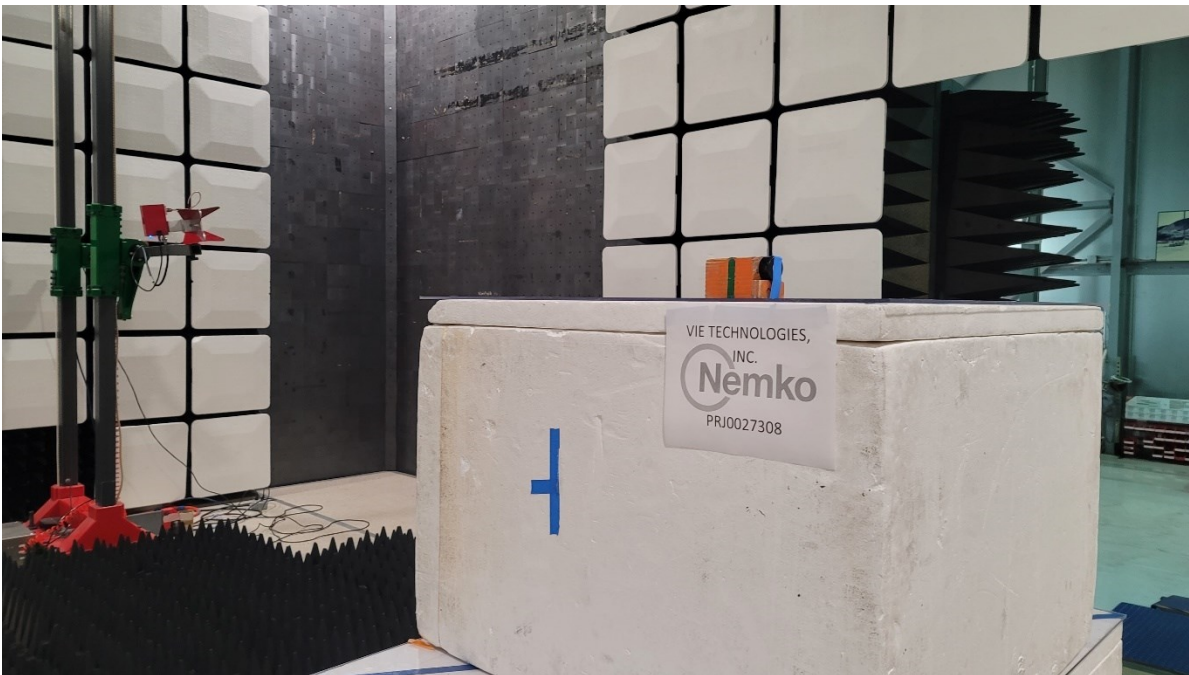
Figure 3 - Radiated emissions above 1 GHz (1-18 GHz).
