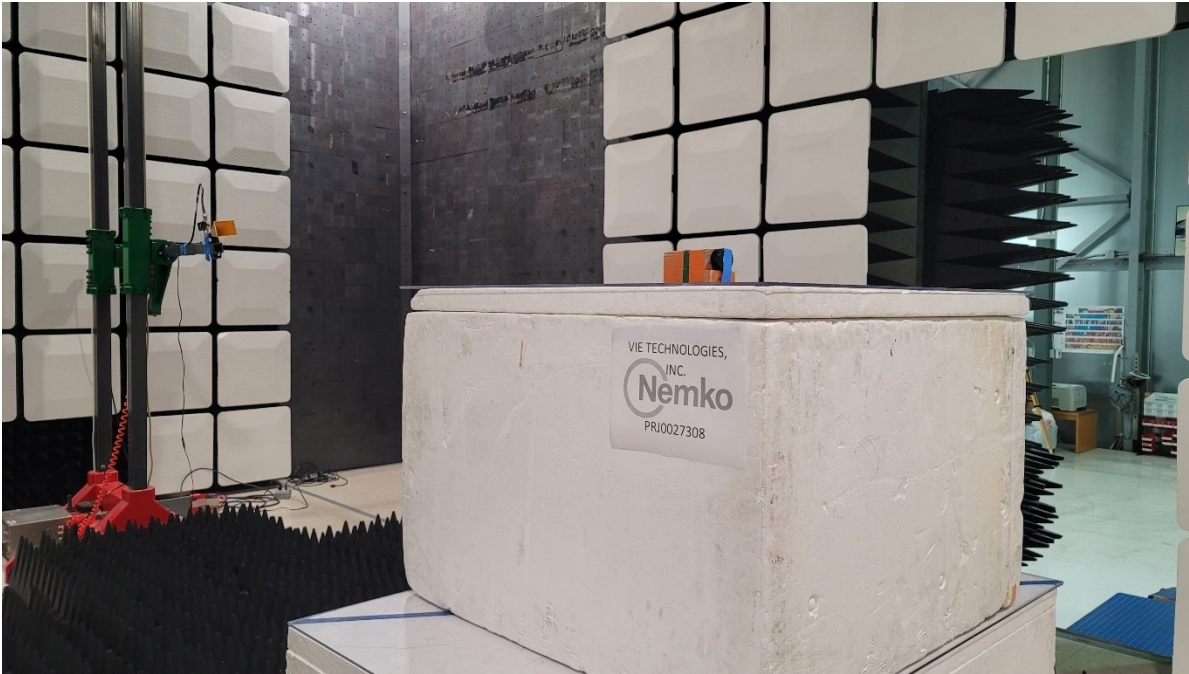
Figure 4 - Radiated emissions above 1 GHz (18-26.5 GHz).
