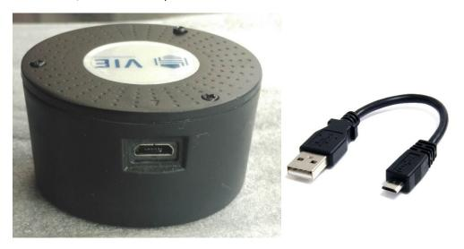
STEP 1: Connect the modified micro USB to USB cable, supplied by VIE Technologies, to the OPA mote.
