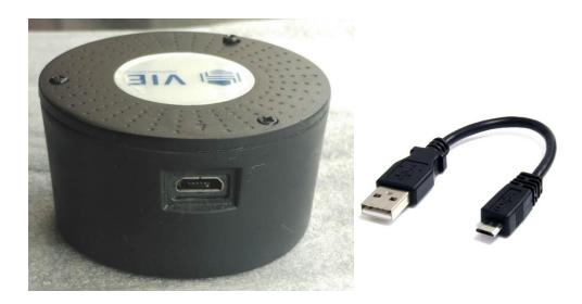
STEP 1: Connect the modified micro USB to USB cable, supplied by VIE Technologies, to the OPA mote.
