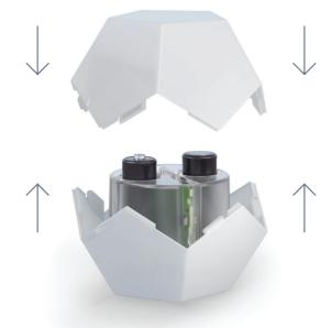
**Note!** After TimeFlip2 switches on, it shall go through a quick (5 sec) self-test, blinking in the following color sequence: red-yellow-green-azure-blue-magenta. After this sequence is complete, TimeFlip2 stops blinking, which means it is ready for use. If the sequence is cut short on red or yellow color, the device is defective.
