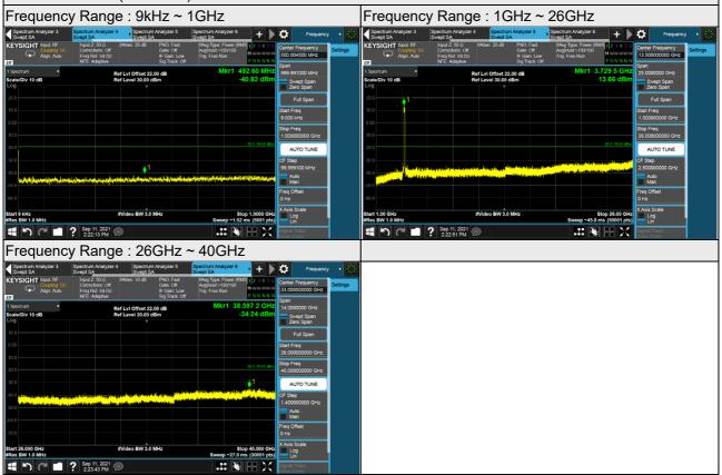
\*The 9 kHz tone is from the spectrum analyzer.
