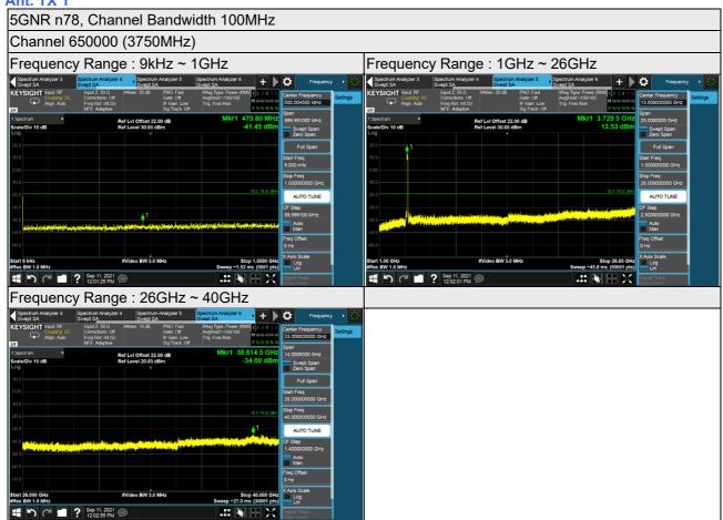
\*The 9 kHz tone is from the spectrum analyzer.
