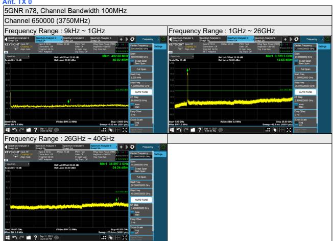
\*The 9 kHz tone is from the spectrum analyzer.
