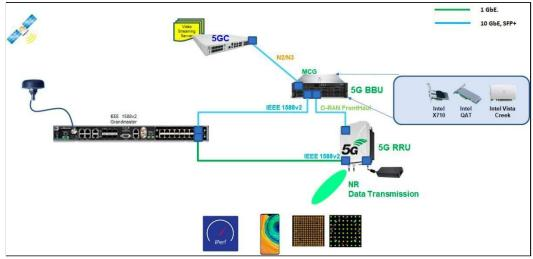
Figure 8 SA L5G System Architecture
