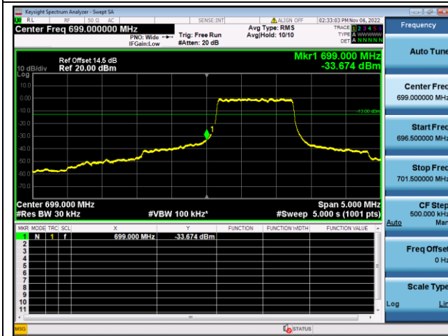
QPSK Low channel-6 RB offset 0
