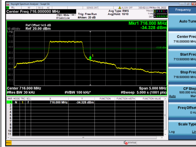
QPSK High channel-6 RB offset 0
