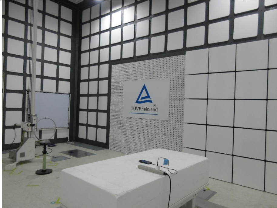
Photograph 28: Test Setup for Spurious Emissions (Back View 2)
