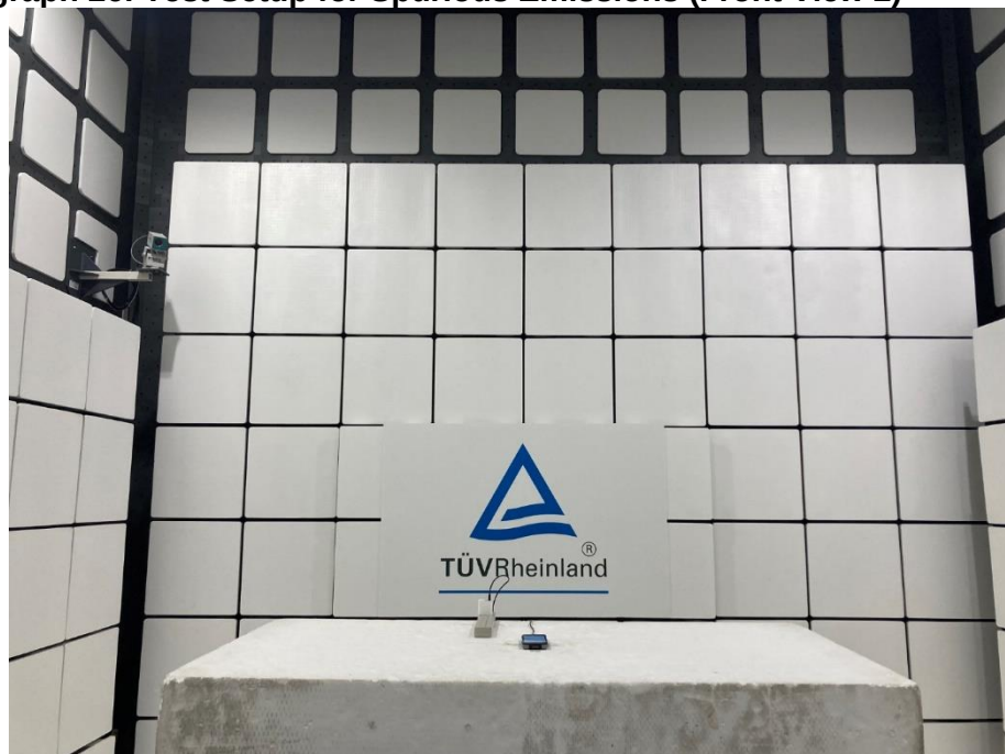
Photograph 26: Test Setup for Spurious Emissions (Front View 2)
