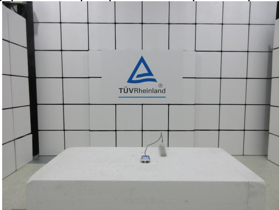
Photograph 44: Test Setup for Spurious Emissions (Front View 1)
