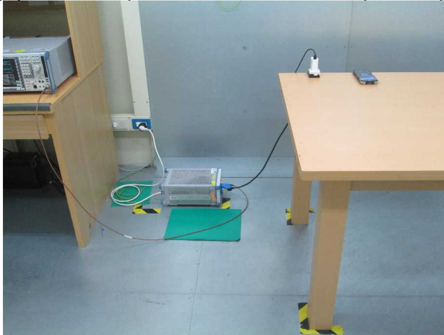
Photograph 50: Test Setup for Mains Conducted Emissions (Back View)
