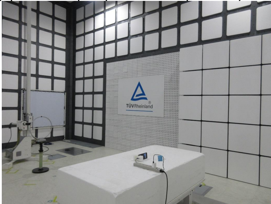
Photograph 16: Test Setup for Spurious Emissions (Back View 2)
