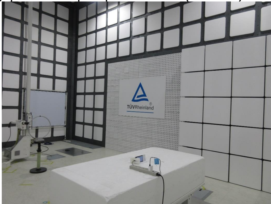
Photograph 32: Test Setup for Spurious Emissions (Back View 1)
