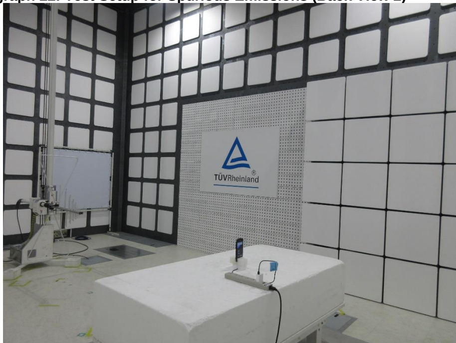
Photograph 22: Test Setup for Spurious Emissions (Back View 2)
