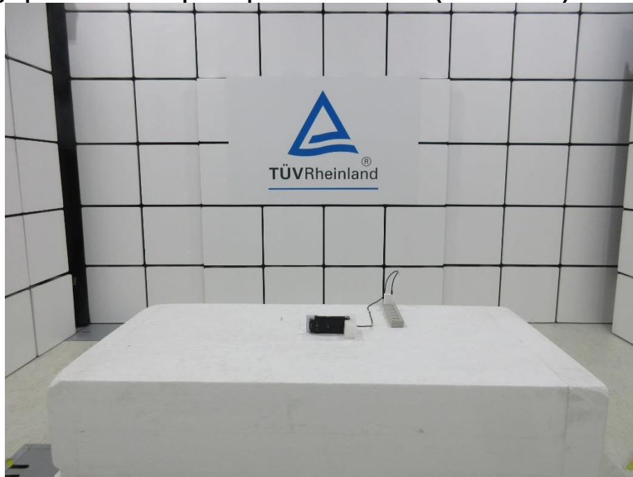
Photograph 34: Test Setup for Spurious Emissions (Front View 1)
