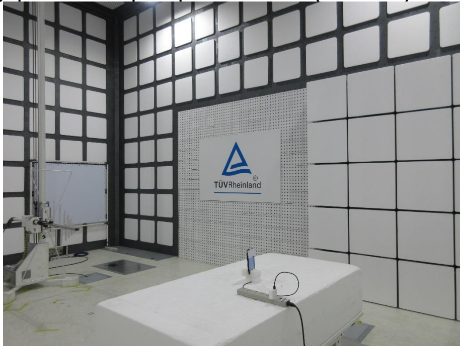
Photograph 42: Test Setup for Spurious Emissions (Back View 2)
