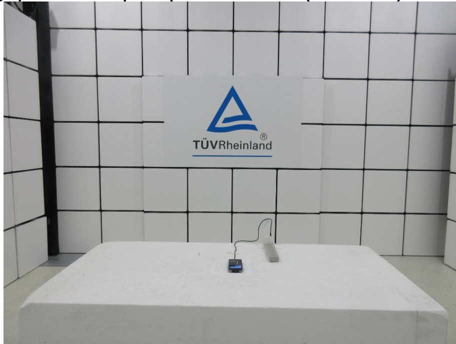
Photograph 7: Test Setup for Spurious Emissions (Front View 1)
