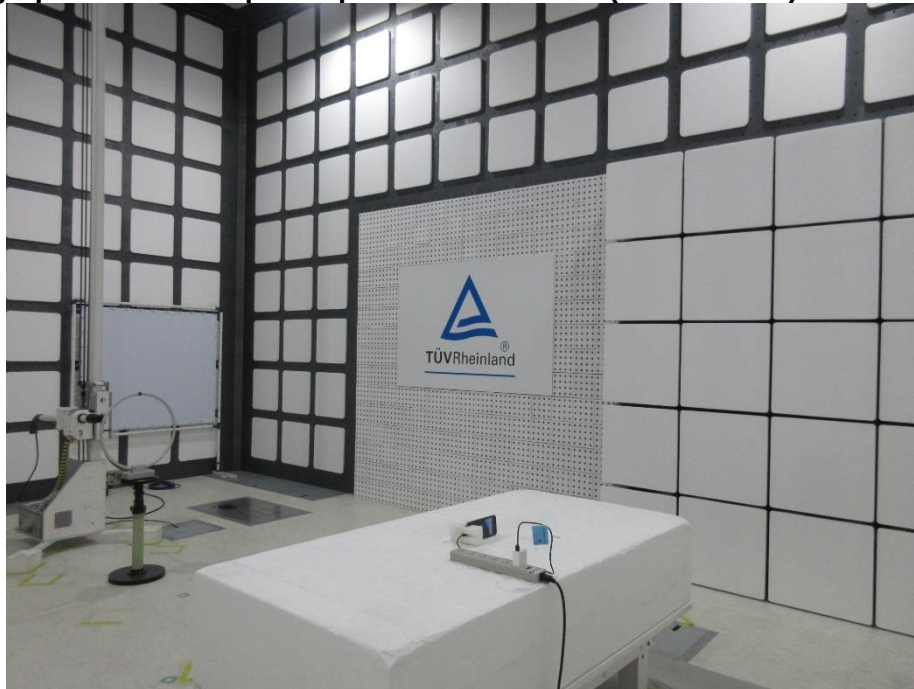
Photograph 4: Test Setup for Spurious Emissions (Back View 2)
