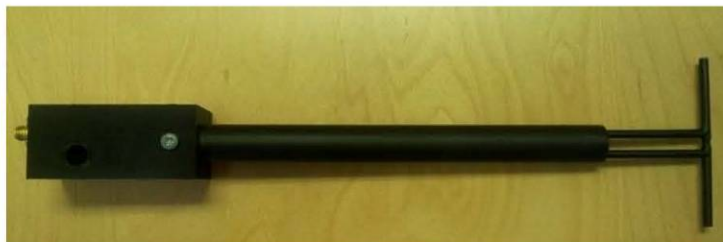
Figure 1 – MVG COMOSAR Validation Dipole
