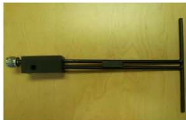
Figure 1 – MVG COMOSAR Validation Dipole
