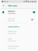
Featuring dual-SIM card slots, the PD470 supports dual-SIM mobile connection, allowing you to enjoy constant and seamless Internet connection. Two cellular network icons will be displayed in the **Status Bar** to indicate the connectivity and signal strength.
