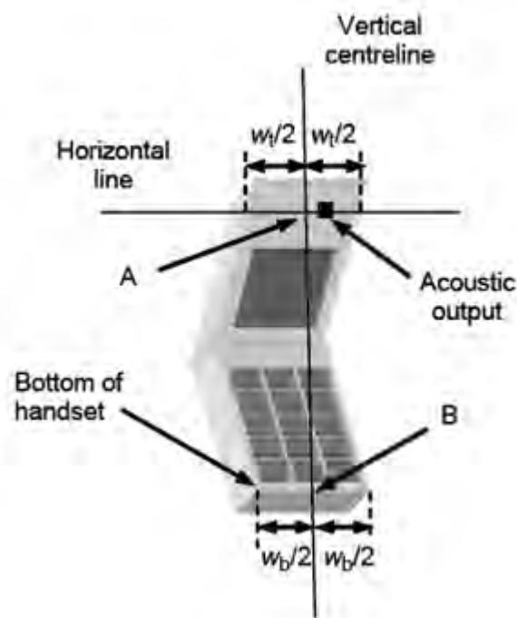
Fig 6.2.2 Handset vertical and horizontal reference lines—"clam-shell case"
