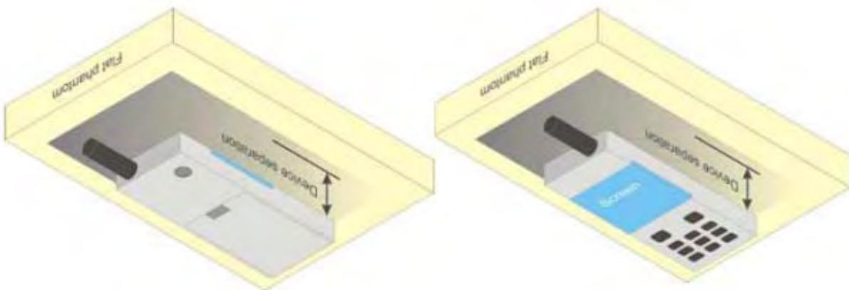
Figure 6.4.1 – Test positions for body-worn devices
