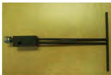
Figure 1 – MVG COMOSAR Validation Dipole
