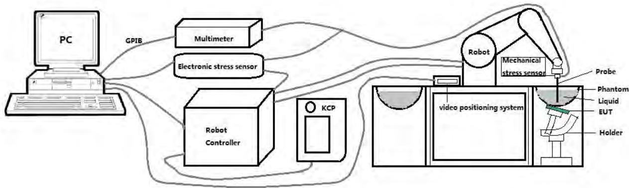
These measurements were performed with the automated near-field scanning system OPENSAR from SATIMO. The system is based on a high precision robot (working range: 901 mm), which positions the probes with a positional repeatability of better than  $\pm 0.03$  mm. The SAR measurements were conducted with dosimetric probe (manufactured by SATIMO), designed in the classical triangular configuration and optimized for dosimetric evaluation.
