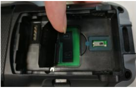
Figure 2-3 Remove the plastic cover.
