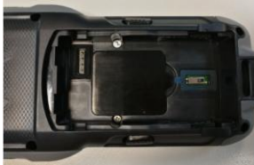
Figure 2-2 Remove the battery
