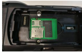
Figure 2-4 As the diagram shown, insert SIM Card and TF Card.
