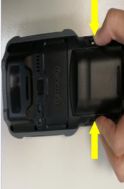
Figure 2-1 Press the two buttons next to the battery.
