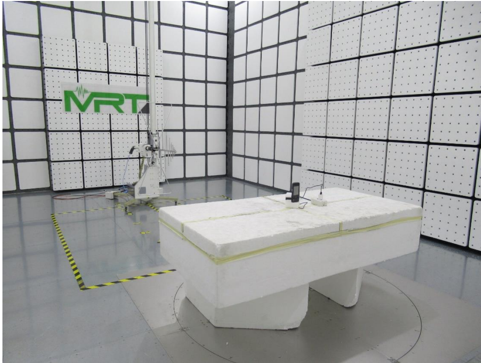
Radiated Emission Test Setup for below 1GHz
