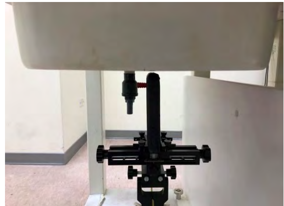
Fig.6 EUT Bottom side to flat phantom
