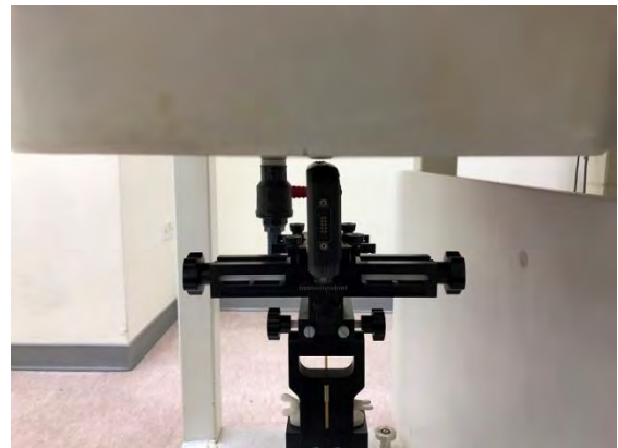
Fig.7 EUT Right side to flat phantom
