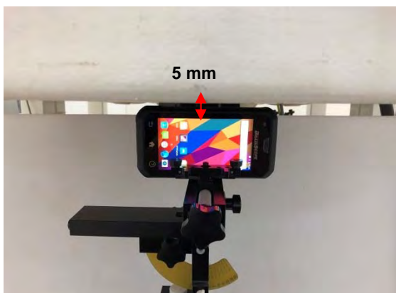
Fig.8 EUT Left side to flat phantom
