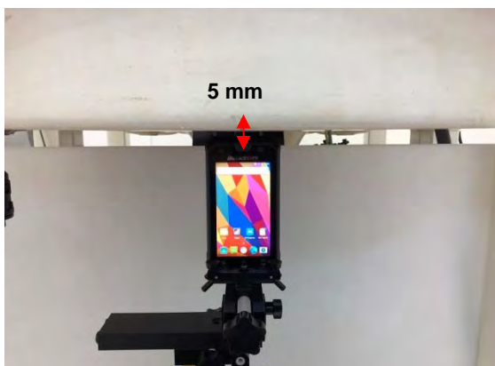
Fig.5 EUT Top side to flat phantom
