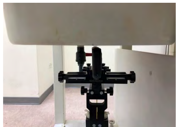
Fig.8 EUT Left side to flat phantom
