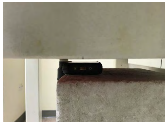
Fig.3 EUT Front side to flat phantom
