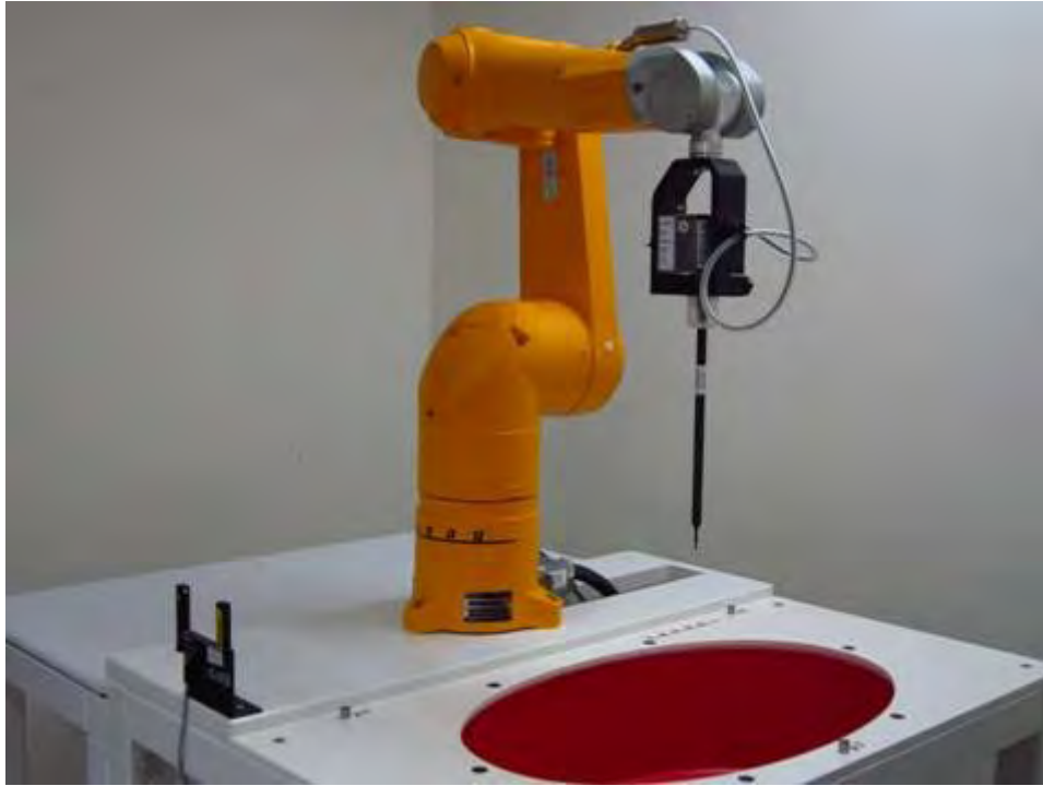
Fig.1 Photograph of the SAR measurement system
