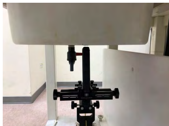
Fig.5 EUT Top side to flat phantom
