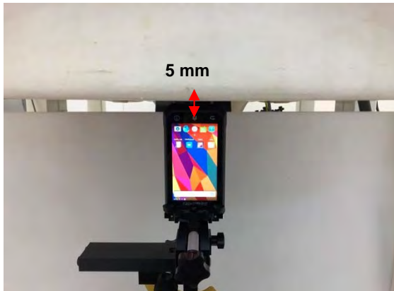
Fig.6 EUT Bottom side to flat phantom
