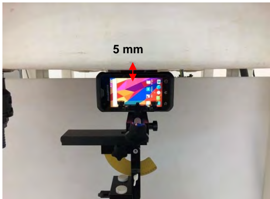
Fig.7 EUT Right side to flat phantom
