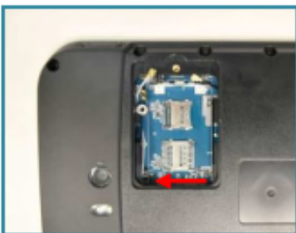
Figure 2-5 Follow the direction of red arrow to open the lid of mSD slot.
