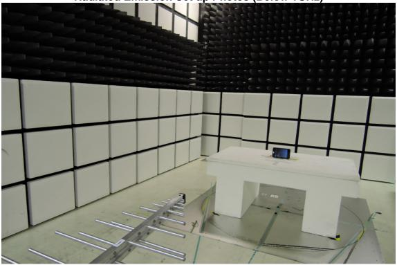
Radiated Emission Set up Photos (Above 1GHz)
