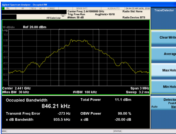
20dB Bandwidth plot on channel 78 (1Mbps)
