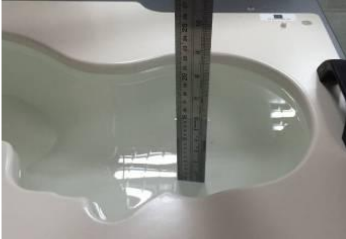
Head Position with 5000MHz liquid depth (15.3cm)
