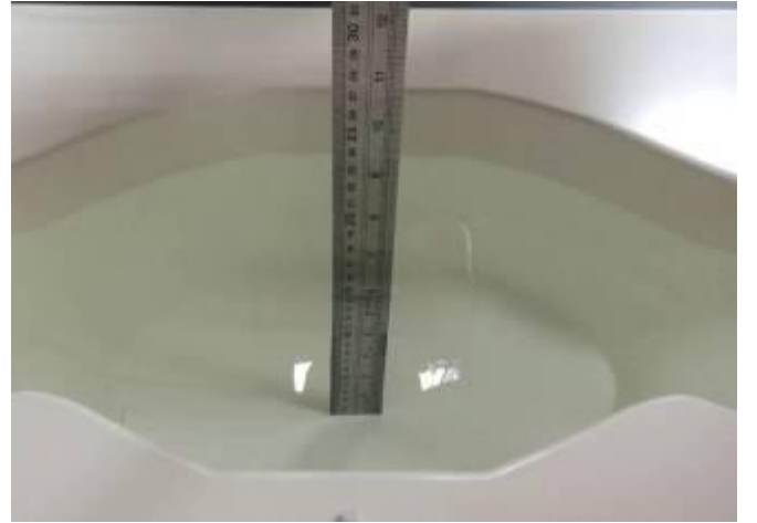
Body Position with 5000MHz liquid depth (15.2cm)
