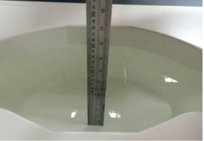
Body Position with 5000MHz liquid depth (15.2cm)
