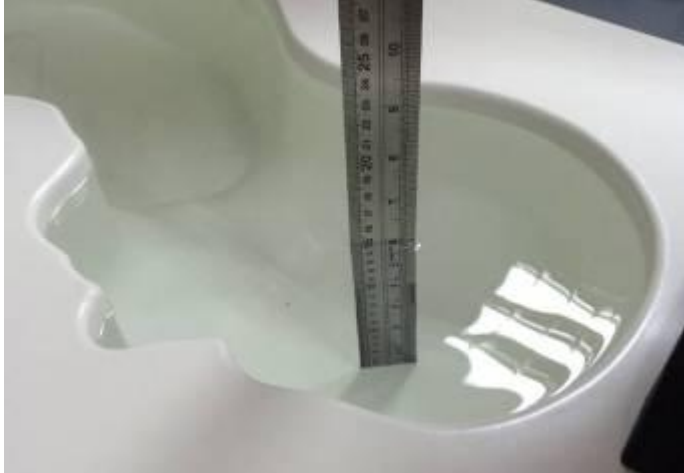
Head Position with 5000MHz liquid depth (15.3cm)
