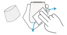
Wipe all accessible surfaces of the device and cap, using moderate pressure, as shown.
