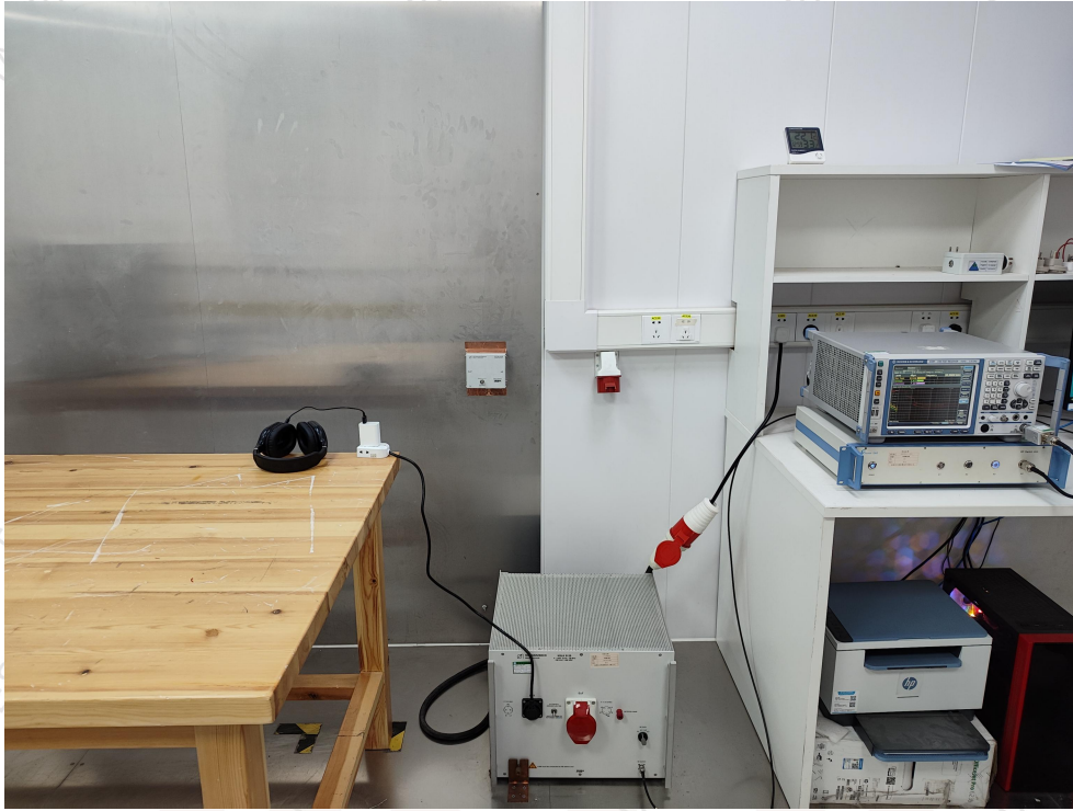
Photo of Conducted Emission Measurement
